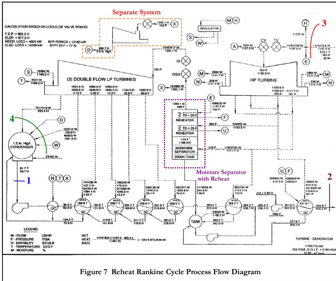
Figure 7 Reheat Rankine Cycle Process Flow Diagram
